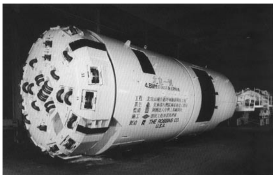
Figure.5 Robbins TBM type 153-269 used for pilot tunnel.
